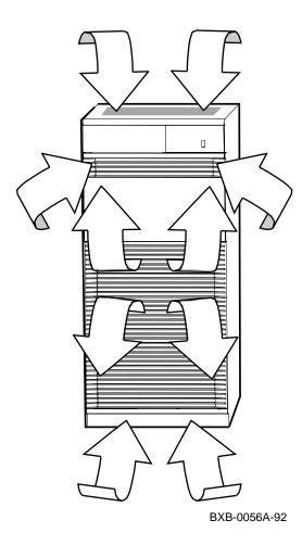
The cooling system is designed to keep system components at an optimal operating temperature. It is important to keep the front and rear doors free of obstructions, leaving a minimum clear space of 1.5 meters (59 inches) in the front and 1 meter (39 inches) in the rear between cabinets to maximize airflow (see Figure 1-1).
