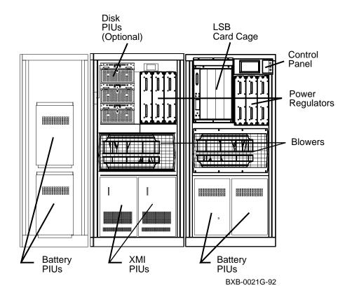
These components are visible from the inside front of the cabinet (see Figure 1-4 for their location):
