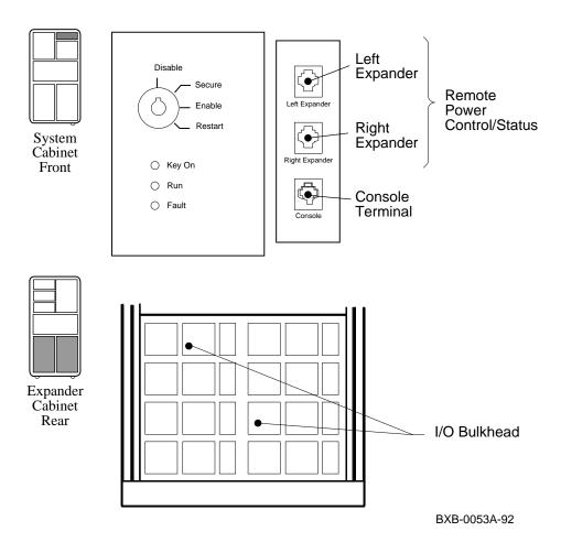
Console terminal I/O and expander cabinet remote power control/status connections are located to the right of the control panel. These three modular jacks allow power control/status connections to the left expander cabinet, right expander cabinet (if present), and I/O connections to the console terminal. The console terminal modified modular jack is keyed so that an expander cabinet connector cannot be plugged into its jack.
