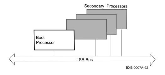
One processor is designated as the boot processor (or primary processor) and becomes the primary communicator to the console terminal.
