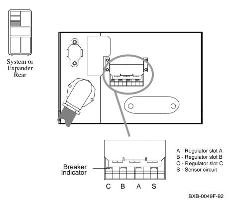
Circuit breakers and power indicators are at the rear of the system and expander cabinets.
