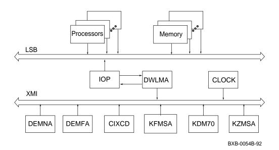
The LSB bus is a synchronous 128-bit system bus that interconnects the processors, memory modules, and the I/O port (IOP) module. The IOP module connects the LSB bus to I/O buses through separate I/O adapter modules.
