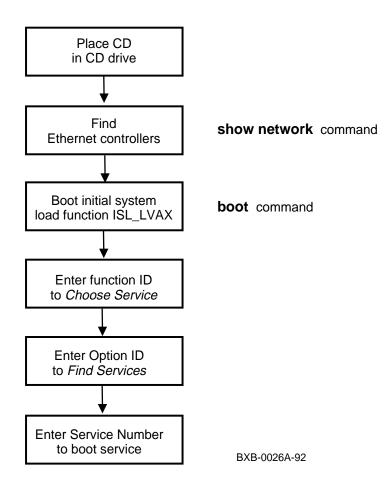
Some systems use Ethernet-based CD servers to load the operating system. The InfoServer consists of one or two CD drives and connects to standard Ethernet or ThinWire groups or networks.
