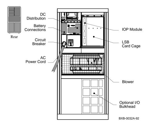
The following components are visible from the rear of the cabinet (see Figure 1-5):
