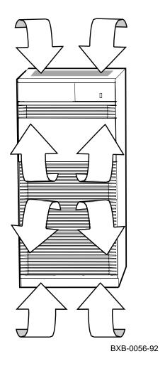
The cooling system is designed to keep system components at an optimal operating temperature. It is important to keep the front and rear doors free of obstructions, leaving a minimum clear space of 1.5 meters (59 inches) in the front and 1 meter (39 inches) in the rear between cabinets to maximize airflow (see Figure 1-1).
