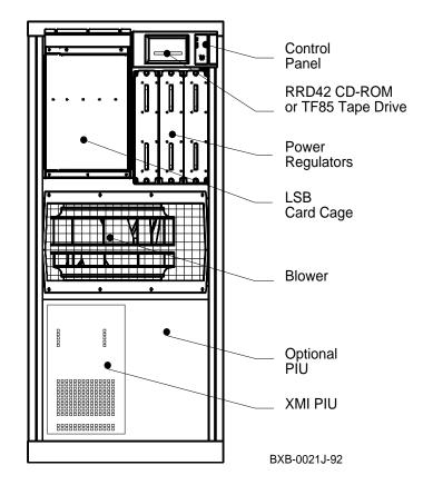
These components are visible from the inside front of the cabinet (see Figure 1-4 for their location):
