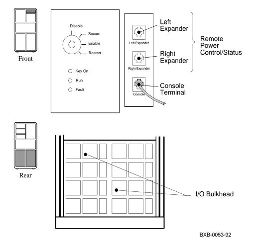
Console terminal I/O and expander cabinet remote power control/status connections are located to the right of the control panel. These three modular jacks, allow power control/status connections to the left expander cabinet, right expander cabinet, and I/O connections to the console terminal. The console terminal modified modular jack is keyed so that an expander cabinet connector cannot be plugged into its jack.
