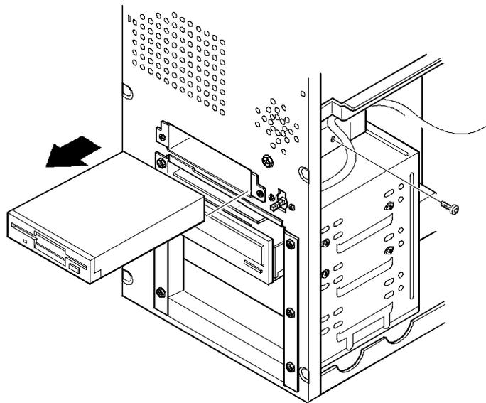
Figure 3 - 6 Removing the 3½-Inch Diskette Drive
