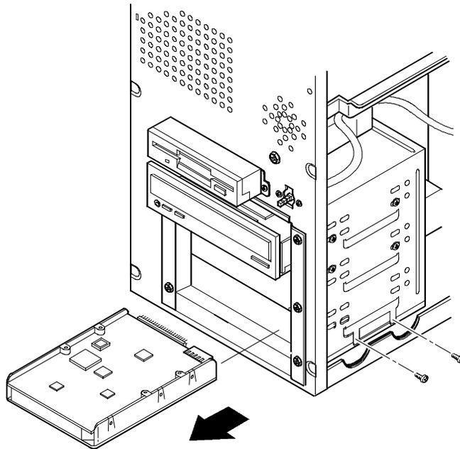
Figure 3 - 8 Removing the IDE Hard Disk Drive
