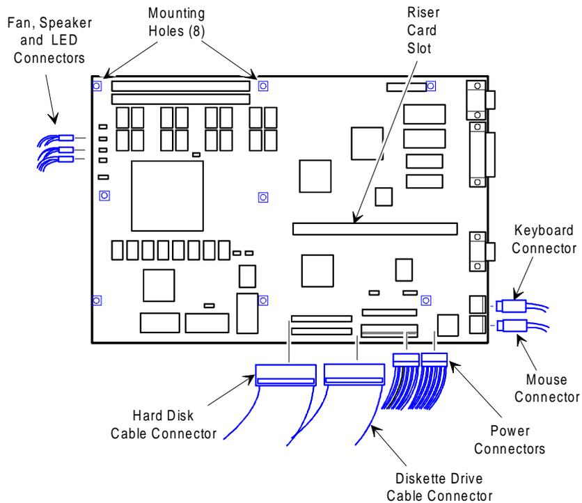
Figure 3 - 10 Removing the Main Logic Board
