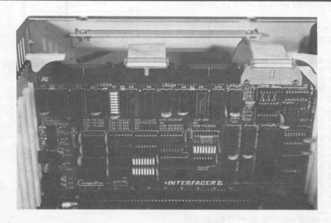
Shown above is a typical installation using (2) optional Interfacer cable assemblies. These cables consist of an Ansley 609-25S 25-pin 'D' connector and an Ansley 609-2601M 26-pin female transistion connector.
