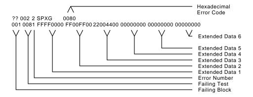
Table A-26 lists the failing logical blocks that display when you enter the SHOW ERROR command. The failing block field points to an area that you can use as a starting point for diagnosing the fault. The error is detected at this point, but is not always the actual fault.
